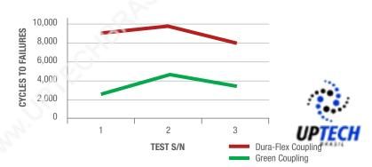
When a new, out-of-the-box, Dura-Flex coupling and a green coupling were subjected to a stop-start cycle test, Dura-Flex was 2X - 100X better.
