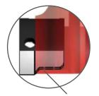
Step profile in shoe. lowers stress which can cause failure at the bonding point.
